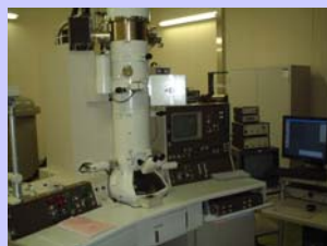
Figure 3. JEOL 2010F: A high-resolution TEM with single-atom sensitivity
