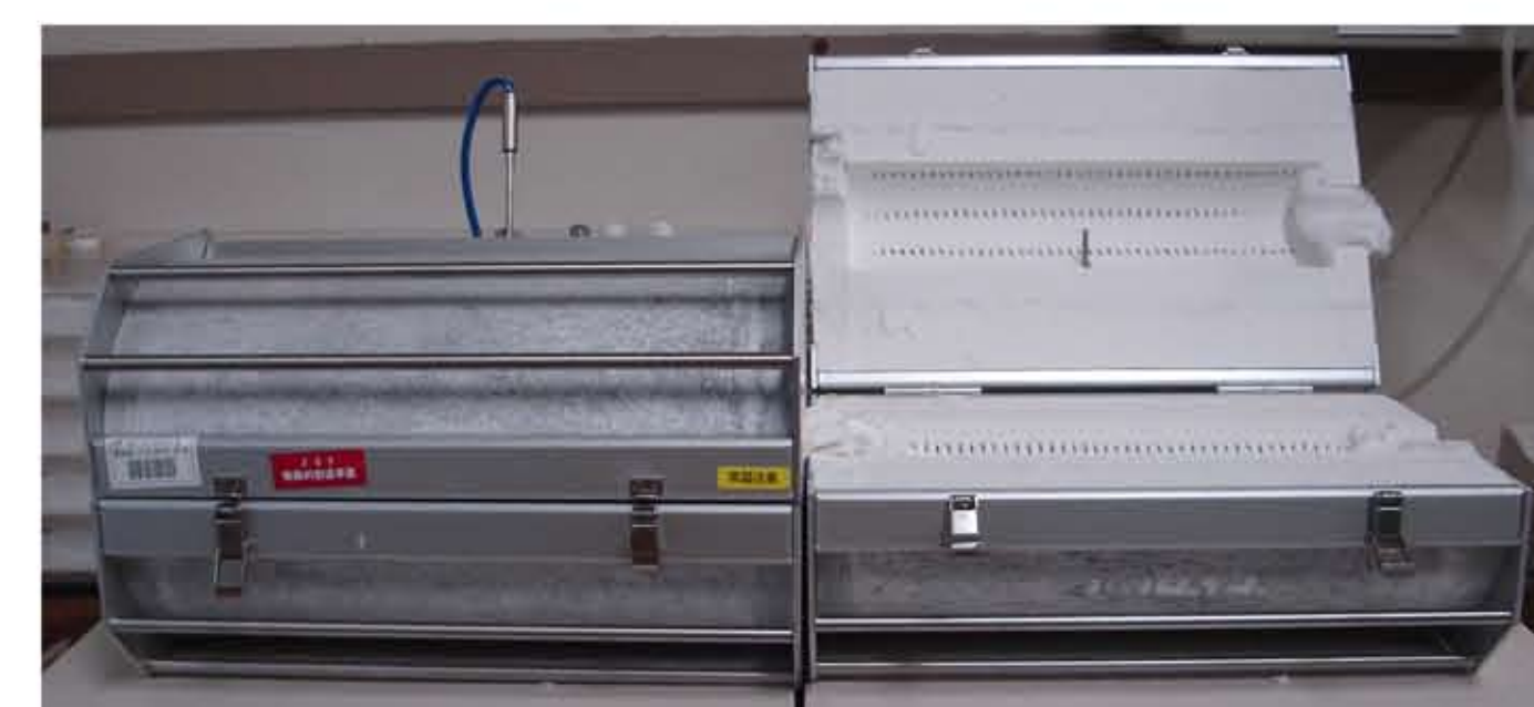
Fig. 2b, Two ovens at T_H and T_C , Insulation gap causes large T drop (see fig. 2d).
