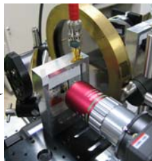
Fig. 3 - A close-up of part of the system. The objective lens, sample, solid immersion lens, parabolic mirrors and polarizer can be seen.
