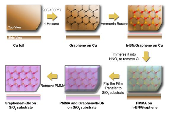
We have also grown h-BN films from ammonia borane with additional ammonia as a reactant to produce nitrogen enriched h-BN. Samples were analyzed with EELS, Raman spectroscopy, AFM, and TEM.
