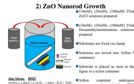
microwave radiation for 3hr at 95°C ZnO NRs have a high aspect ratio which allows optimal immobilization due to a high surface area to volume ratio. The demonstrated ZnO low temperature growth of NRs is a very promising method for integration of biosensors. Previously low temperature, selective growth has been demonstrated.
