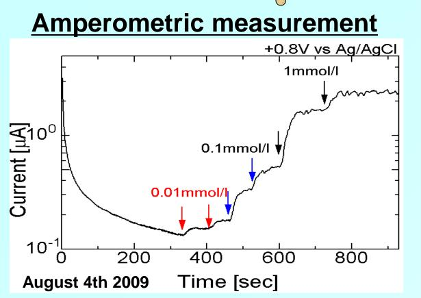
This graph shows a successful sensing test. The current reading steps up after addition of glucose, the greater the concentration the higher the step.
