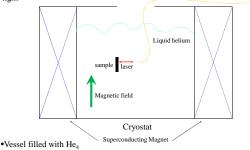
•Maintains cryogenic temperatures for experiments
