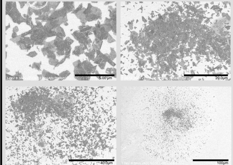
High concentrations of graphene were observed on the SEM.
