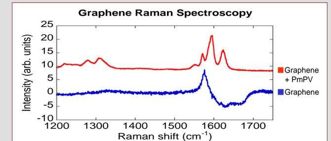
Raman Analysis further characterized the graphene with a peak intensity at 1580  $\text{cm}^{-1}$  as usually seen.
