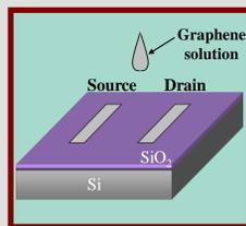
SWCNT can be printed in random networks to create Field Effect Transistors.
