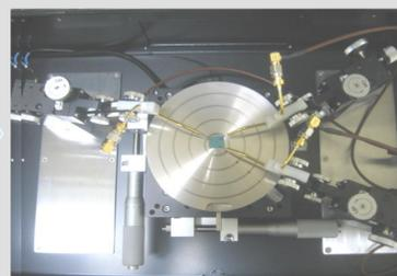
(Transistor Parameter Analyzer and substrate)
