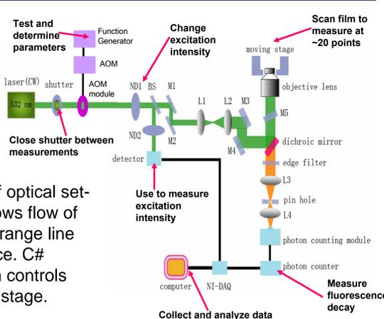
(Right) Diagram of optical set-up. Green line shows flow of excitation laser. Orange line shows fluorescence. C# computer program controls shutter, ND1, and stage.
