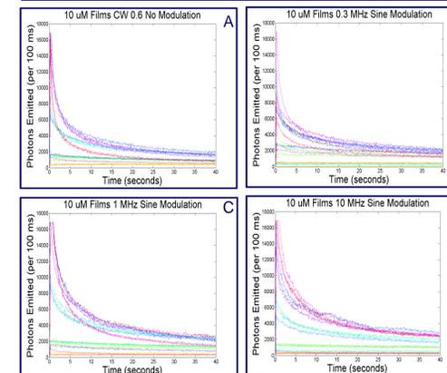
(Left) Fluorescence vs. time graphs for 4 modulation conditions. (A) CW no modulation. (B) 0.3 MHz sine modulation. (C) 1 MHz sine modulation. (D) 10 MHz sine modulation. Comparing (A) and (C) shows that sine modulation at 1 MHz gives a slower decay rate when compared to no modulation case.
