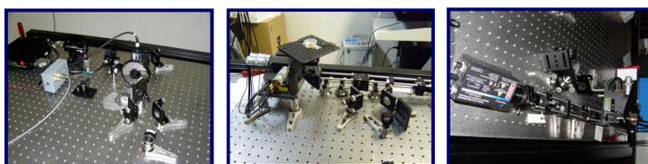
Experimental Optical Set-Up: (Left) excitation laser, shutter, ND filter, and detector to measure excitation intensity. (Middle) scanning piezoelectric stage and dichroic mirror. (Right) photon counting module collecting fluorescence from sample and objective lens.
