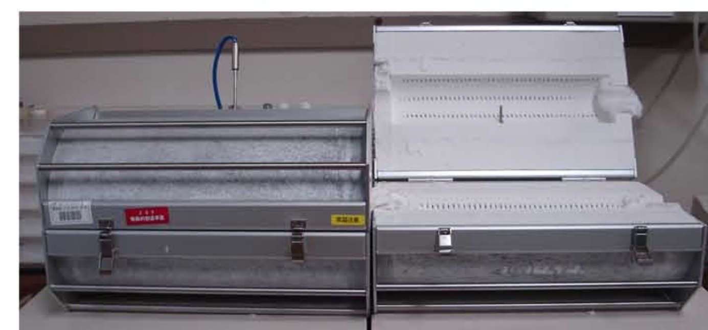
Fig. 2b, Two ovens at T_H and T_C , Insulation gap causes large T drop (see fig. 2d).
