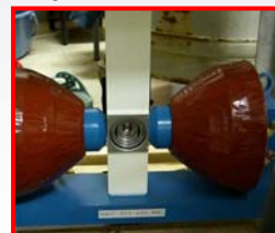
Sample in cryostat with magnets on either side
